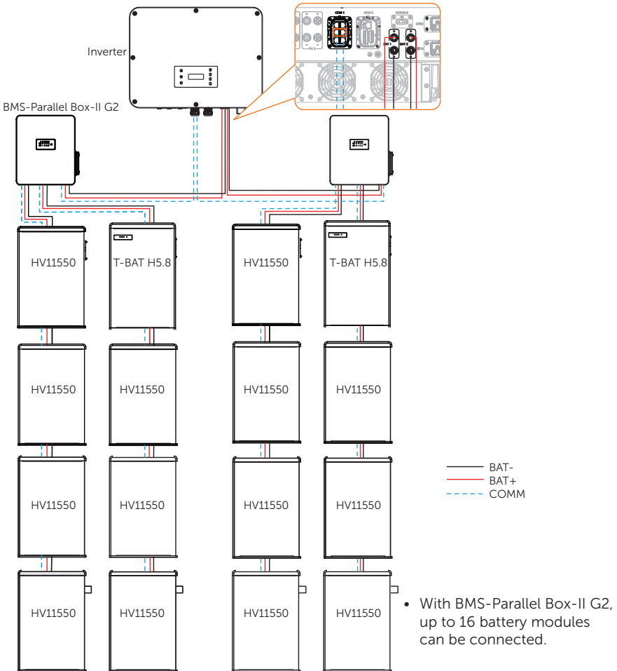
Figure 8-26 Battery connection with BMS-Parallel Box-II G2
